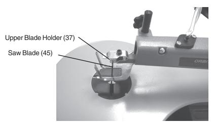
The Scroll Saw can use a variety of blade widths and thicknesses, as long as they are five inches long and have the cross pin for mounting. These are used for cutting various types of materials as listed below:
